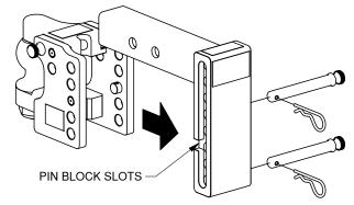
Figure 5: Replacing pintle hook.
