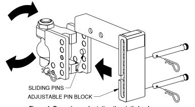
Figure 4: Removing and rotating the pintle hook.
